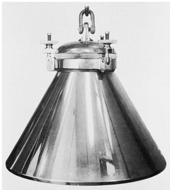
Fig. 4. “Korbnetz”, Hensen’s device used with conical net. One of the many inventions by Victor Hensen to collect plankton. Photo: P. Roggero. Souce: National Oceanic and Atmospheric Administration.
